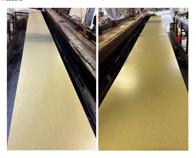
**Photograph No. 1:** Test specimen prior to testing showing the entire 24-foot test specimen from the fire exposure chamber's burner end (left), and vent end (right).
