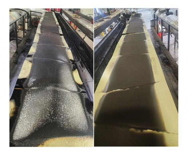
**Photograph No. 2:** Test specimen from the test chambers burner end (left), and vent end (right) showing the post 10-minute test sample condition immediately after removal from the test chamber.
