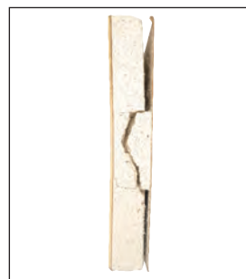
Rigid plastic wall covering failed.
