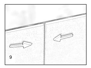
Artizan Max FRP Panels can be applied using Division Trim or, to maximize visual appeal, using a panel-to-panel joinery method. Each Artizan Max panel is factory cut square on all four sides to ensure a more seamless appearance by sliding the panels flush together.
