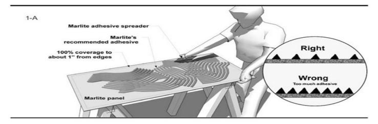
Use Marlite brand C-551 FRP Adhesive (sub wall must be porous) or the Advanced Polymer Adhesive to satisfy low VOC requirements
