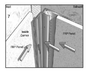
For high moisture areas, apply a continuous bead of silicone sealant in the corner and in the Inside Corner Trim Molding channel. Secure Inside Corner Trim Molding to cover bead. (see illustration 7)
