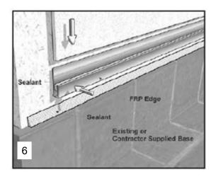
Curb must be installed first. For high moisture areas, apply a continuous bead of silicone sealant to the top of curb or floor line and in the Trim Molding channel. Set Edge Trim Molding in place and fasten to the sub wall. Slip FRP Panel into Edge Trim Molding. Execute similar application at ceiling line. (see illustration 6)
