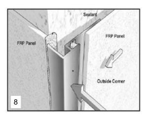
First, cut the FRP Panel on the preceding wall flush to the outside corner and install. For high moisture areas, apply a continuous bead of silicone sealant to both Outside Corner Trim Molding channels. Secure into place and slip in the next FRP Panel. (see illustration 8)
