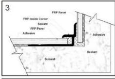
Where steam cleaning is required, and high moisture conditions are prevalent; all Trim Molding and FRP Panels must be sealed with Marlite brand Silicone Sealant to ensure a watertight seal. (see illustrations 3-5)
