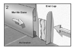
Apply ¼" bead of Marlite brand Silicone MS250 Clear Silicone Sealant to top, face and bottom of End Cap. Attach End Cap to Base Molding. A sufficient amount of sealant must be applied, creating some "squeeze out" ensuring a moisture proof seam when End Cap is applied to the Base Molding. (see illustration 2)
