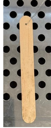
Photo 2. Control (Untreated White Birch Tongue Depressor) after 4 weeks exposure.
