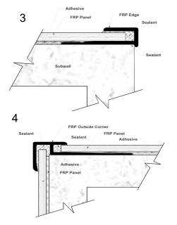
Silicone Sealant is best applied to Trim Molding prior to application to the wall. It is important that a continuous, non-broken bead of sealant is applied. Excess sealant "squeeze-out" should be promptly cleaned off with mineral spirits. It is suggested that a sealant be applied to all exposed edges of molding, electric plates and other covers after installation. Allow 24 hours drying time for sealant. Rough cut Artizan<sup>™</sup> Max FRP Panel edges can be smoothed with sandpaper or a file.
