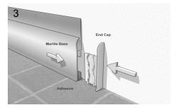
Apply ¼" bead of Marlite brand Silicone MS250 Clear Silicone Sealant to top, face and bottom of End Cap. Attach End Cap to Base Molding. A sufficient amount of sealant must be applied, creating some "squeeze out" ensuring a moisture proof seam when End Cap is applied to the Base Molding. (see illustration 3)
