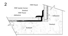
Where steam cleaning is required, and high moisture conditions are prevalent; all Trim Molding and FRP Panels must be sealed with Marlite brand Silicone Sealant to ensure a watertight seal. (see illustrations 2 - 4)
