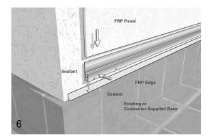
Curb must be installed first. For high moisture areas, apply a continuous bead of silicone sealant to the top of curb or floor line and in the Trim Molding channel. Set Edge Trim Molding in place and fasten to the sub wall. Slip FRP Panel into Edge Trim Molding. Execute similar application at ceiling line.
