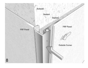
First, cut the FRP Panel on the preceding wall flush to the outside corner and install. For high moisture areas, apply a continuous bead of silicone sealant to both Outside Corner Trim Molding channels. Secure into place and slip in the next FRP Panel. (see illustration 8)
