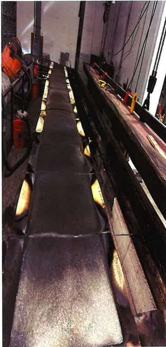
Photograph No. 2: Test specimen from the test chambers burner end (left), and vent end (right) showing the post 10-minute test sample condition immediately after removal from the test chamber.
