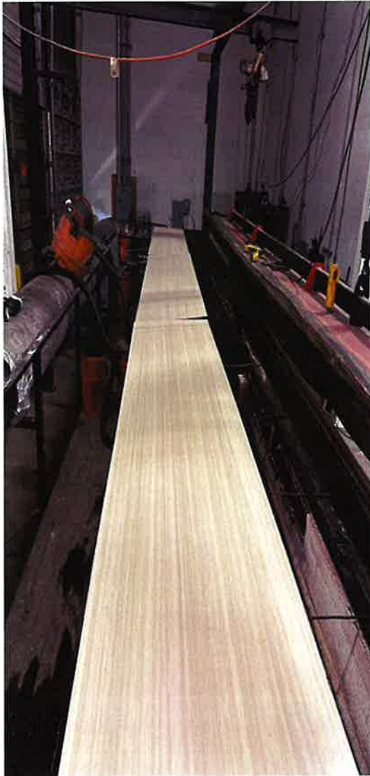
Photograph No. 1: Test specimen prior to testing showing the entire 24-foot test specimen from the fire exposure chamber's burner end (left), and vent end (right).
