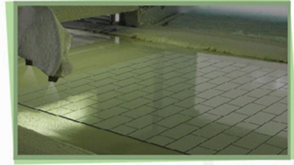
Marlite's Sani-coat sealer is spray applied to add that extra layer of durability, plus stain and mildew resistance.
