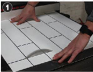
FRP Panels are easily trimmed on a table saw.
