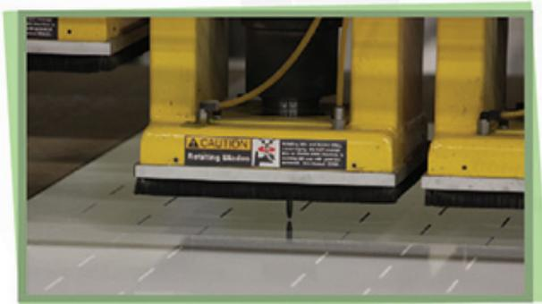
Cutting-edge CNC technology grooves Symmetrix™ FRP panels with extreme precision, ensuring every panel has a seamless fit and appearance.
