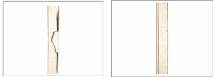
Rigid plastic wall panel Complete structural failure
