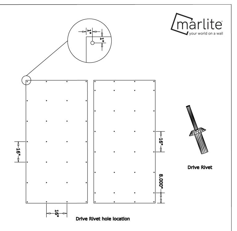
Pre-drill 9/32" hole, which is slightly over-sized to allow for panel expansion. Remove any excess debris or dust from hole. Insert rivet snug to panel face. Lightly tap in pin head using a flat-faced hammer. This will cause the Pin Body to expand. Stagger fastening points on adjacent panels. Typically 28-32 fastners per panel.
