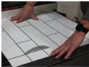
FRP Panels can be easily cut with a table saw.
